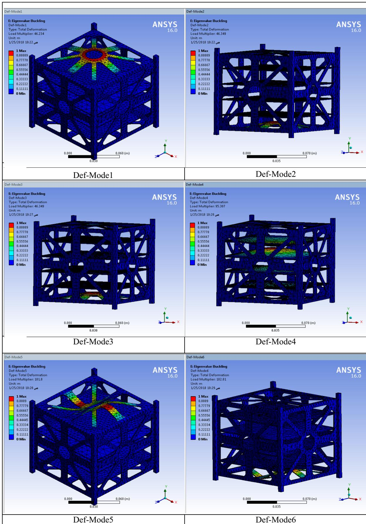
Fig. 1. Total Deformation and Buckling modes for Al-7075 structure.
